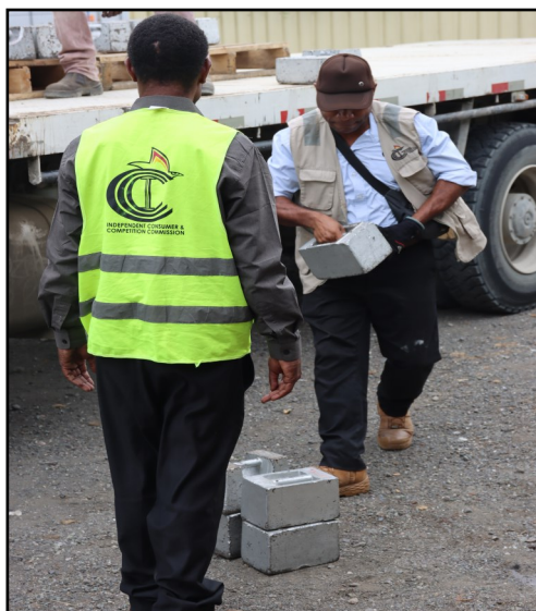
Top left: An officer weighing a 5kg weight on a scale at PNG LNG site. Right: 20kg weights were used to test the scale capacity at 100kg at the Pacific Helicopters office site in Port Moresby.
