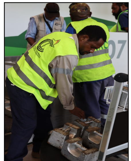
Top left: An officer weighing a 5kg weight on a scale at PNG LNG site. Right: 20kg weights were used to test the scale capacity at 100kg at the Pacific Helicopters office site in Port Moresby.
